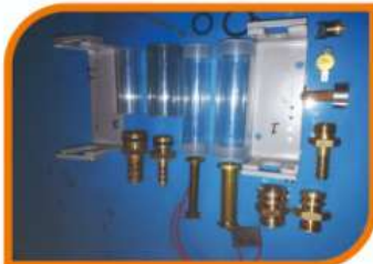
Flow Switch And Components
