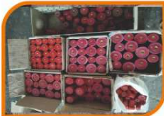
Bus Bar Supporter Insulator
