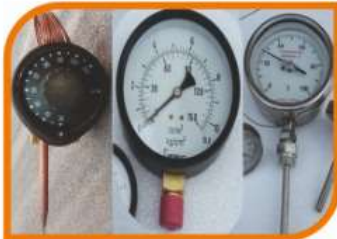
Pressure Switch, Pressure Gauge, Temperature Gauge
